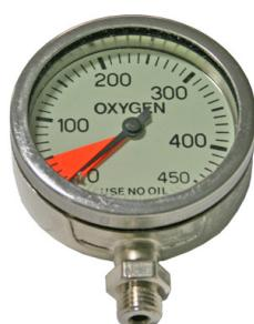
High-quality brass pressure gauge, suitable especially for main tanks and stages. Synoptic dial scale up to 450 bar. Suitable and marked for oxygen use. Comes with swivel with viton o-rings.
