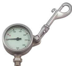
High-quality brass pressure gauge, suitable especially for main tanks and stages. Synoptic dial scale up to 360 bar. With attachment point for different mountings, comes with Shackle Bolt Snap. Comes with swivel with viton o-rings.
